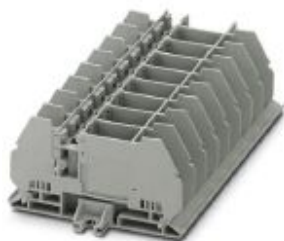
Feed-through terminal block with bolt connection, cross section: 0.1 - 6 mm 2 , AWG: 26 - 10, width 16.3 mm, color: Gray
