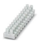
Polypropylene Europe terminal strip, white, for connecting solid conductors and stranded conductors with and without ferrules with a cross section of 0.75 to 6 mm²
