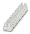
Polyamide Europe terminal strip, transparent, with wire protection, for connecting solid conductors and stranded conductors with and without ferrules with a cross section of 1 to 6 mm²
