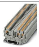
Feed-through terminal block, nom. voltage: 800 V, nominal current: 24 A, connection method: Push-in connection, number of connections: 3, cross section: 0.14 mm² - 4 mm², AWG: 26 - 12, width: 5.2 mm, height: 35.2 mm, color: gray, mounting type: NS 35/7,5, NS 35/15
