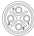
Pin assignment of M12 socket, 4-pos., S-coded, view of socket side
