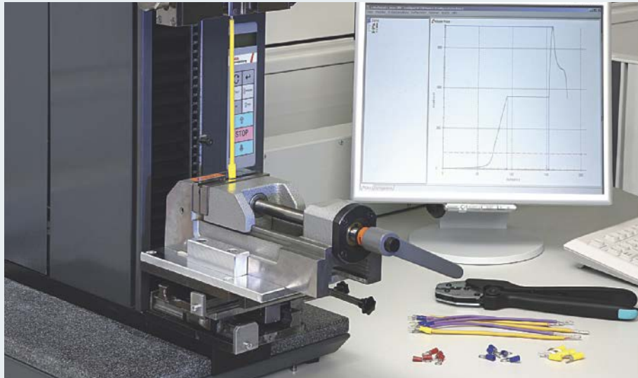
Conductor pull-out test
