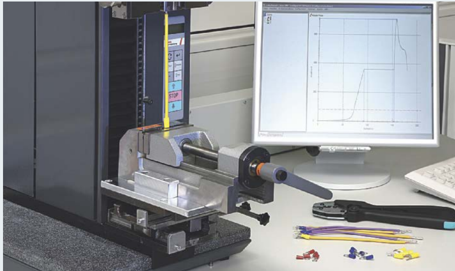
Conductor pull-out test
