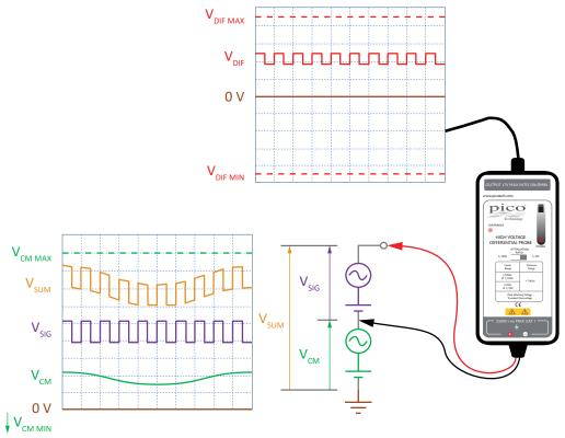
Figure 2 - Using an active differential probe
