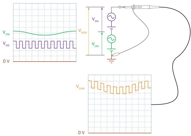
Figure 1 - Using a single-ended oscilloscope probe
