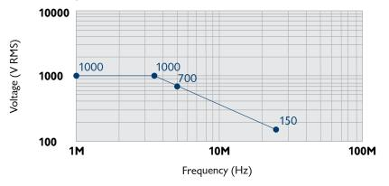
In the example above, the absolute maximum voltage on either of the inputs at low frequencies is 1000 V RMS. At about 3.3 MHz the voltage starts to decline, until at about 25 MHz it is only 150 V RMS. In practice this is seldom a limitation as high frequency and high voltage are rarely found together – such signals being more challenging to generate than they are to measure.
