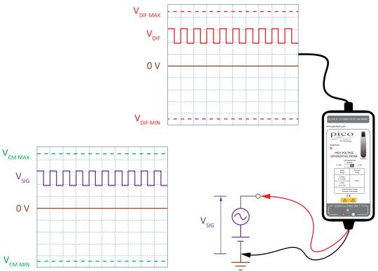
Figure 3 - Single-ended measurement
