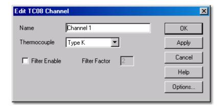
9. From the **Thermocouple** drop-down list, select the type of thermocouple you are using and click **OK.**
