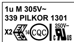
Marking on the top(C ≤ 1uF)
