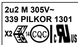
Marking on the top(C > 1uF)
