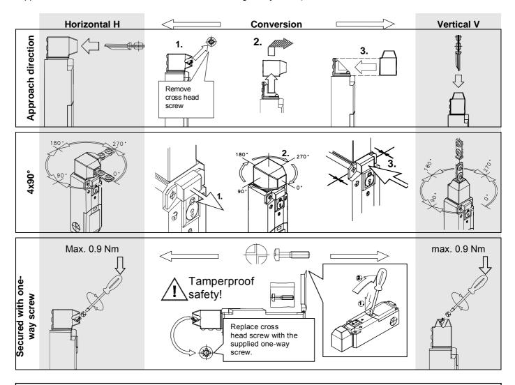
Excess of the maximum torque of 0.9 Nm or installing the actuator so that it is subject to lateral forces may damage the actuating mechanism of the switch gear. This can render the personal protection function useless and cause serious injury or accidental death. Never use the safety switch and actuator as an end stop!
