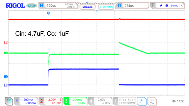
V_{IN}=4.3V , V_{OUT}=3.3V I_{OUT}=1mA to 300mA
