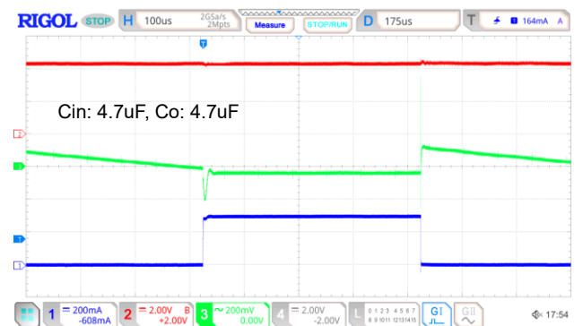
V_{IN}=4.3V , V_{OUT}=3.3V I_{OUT}=1mA to 300mA
