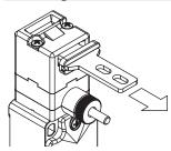
The inside of each switch features a device which holds the actuator in its closed position. Ideal for all those applications where several guards are unlocked simultaneously, but only one is actually opened. The device keeps all the unlocked guards in their position with a retaining force of approx. 30 N, stopping any vibrations or gusts of wind from opening them.
