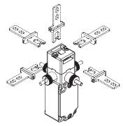
The head can be quickly turned to each of the four sides of the switch by unfastening the two fastening screws
