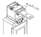
This switch has a wide backlash of the actuator into the head (4,5 mm) to avoid that door gaskets keep in traction the actuator on the solenoid. With closed door, check that the actuator doesn't knock straight against the head of the switch; it must be in the adjustment zone (0,5...5 mm)
