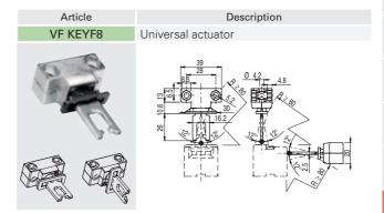
Joined and two directions adjustable actuator for doors with reduced dimensions. The actuator has two couples of fixing holes and it is possible to rotate the actuator-working plan (see picture).
