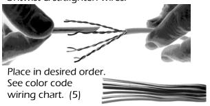
3. Trim wire ends so all conductors are equal length and uniform. Use built in wire cutter in EZ-RJ45<sup>®</sup> Crimp Tool.
