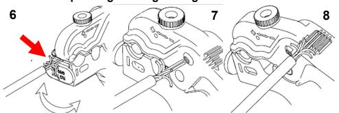
**6.** Grip the ends of a pair using the serrated teeth inside the front end of the tool (see red arrow in Fig 6)
