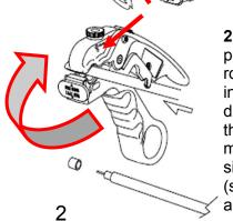
2. For best performance, rotate stripper in same direction as the arrow molded on side of tool (see red arrow)
