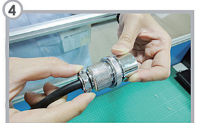
4 半月邊壓入（與線材不能留有間隙） Crescent-shaped clamp mounted (The gap couldn't be allowed with the cable connected)
