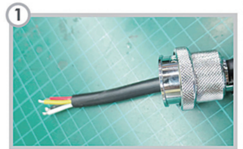
1 線材穿過本體 Cable goes through the body
