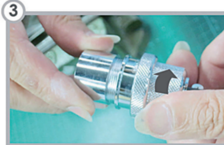
3 本體與上固定體對鎖，將螺紋順時針方向鎖緊（需轉動本體鎖入，非轉動接頭） The body and the upper one are locked together. Screw clockwise and be sure to only rotate the body itself instead of the whole connector
