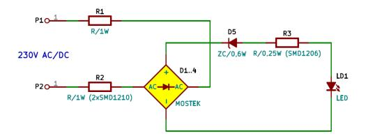
For 24V-AC/DC voltage, power consumption is 0,6 W and for 230V-AC/DC, it is 0,9 W.
