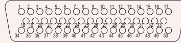
WD 50 Currently available with female contacts. For male contact variants, see page 21.
