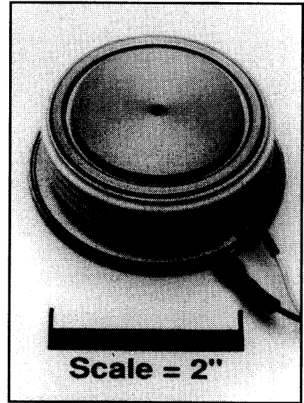
C451 Phase Control SCR 1500 Amperes Average, 2400 Volts
