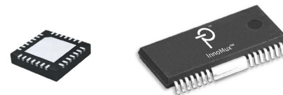
Figure 2. Left – InnoMux in QFN-28, Reflow Process. Right – InnoMux in HSOP-28, Wave Solder Process.
