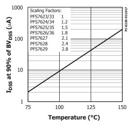
Figure 24. Typical Temperature Dependence of  $\rm I_{\rm DSS}$  at 90% of BV<sub>DSS</sub>.
