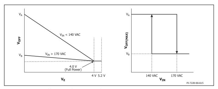
Figure 10. EcoSmart Frequency Slide  $V_{\rm OFF}$  vs.  $V_{\rm E}$  and  $V_{\rm OFF(MAX)}$  vs. Input Voltage.
