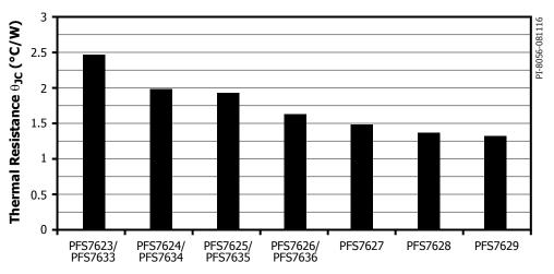
Figure 19. Thermal Resistance eSIP-16D / eSIP-16G Package (  $\theta_{\rm JC}$  ).
