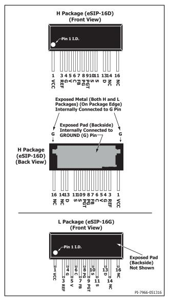
Figure 3. Pin Configuration.
