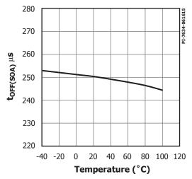
Figure 22.  $t_{OFF(SOA)}$  vs. Temperature.
