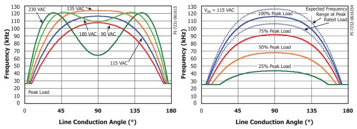
(a) Frequency Variation over Line Half-Cycle as a Function of Input Voltage (b) Frequency Variation over Line Half-Cycle as a Function of Load. Note: Frequency Profiles Shown were Analytically Derived and Reflect CCM Operation Across the Entire Line Cycle.
