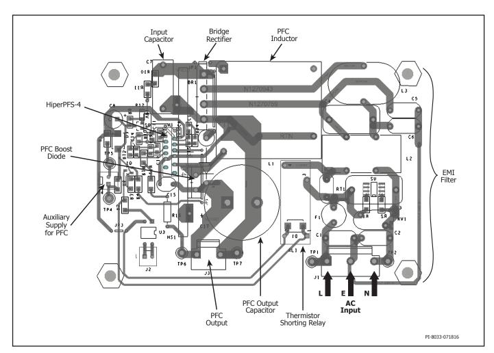
Figure 18. PCB Layout Example.
