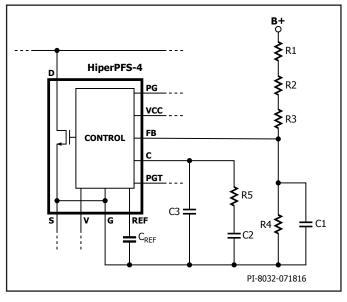
Figure 14. Recommended Feedback Circuit.
