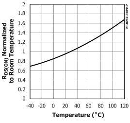
Figure 21.  $R_{DSON}$  vs. Temperature.
