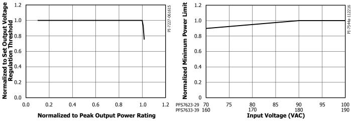
Figure 6. Typical Normalized Output Voltage Characteristics as Function of Normalized Peak Load Rating.
