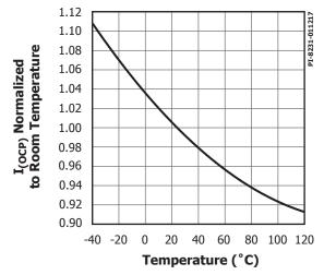
Figure 20.  $I_{(OCP)}$  vs. Temperature.
