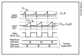
Figure 5. Idealized Converter Waveforms.
