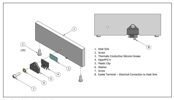
Figure 17. Heat Sink Assembly – with Plastic Clip.
