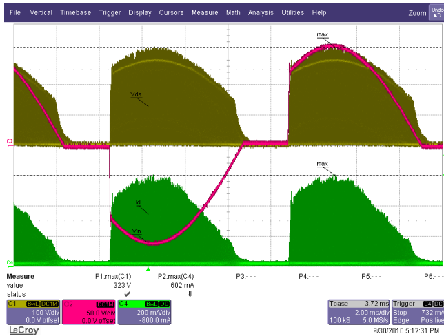
Figure 35 – 115 VAC / 60 Hz, 45° Dimming Phase Angle. 6 LED in Series (18.2 V / 350 mA). Ch1(Yellow): V_{DS} , 100 V / div. Ch2(Red): V_{IN} , 50 V / div. Ch4(Green): I_{DS} , 200 mA / div., 2 ms / div.
