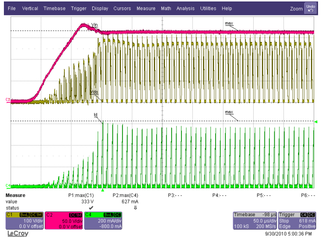
Figure 38 – 115 VAC / 60 Hz, 90° Dimming Phase Angle. 6 LED in Series (18.2 V / 350 mA) Ch1(Yellow): V_{DS} , 100 V / div. Ch2(Red): V_{IN} , 50 V / div. Ch4(Green): I_{DS} , 200 mA / div., 50 μs / div.
