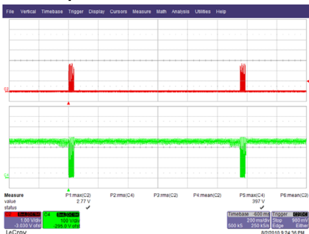
Figure 40 – 265 VAC 60 Hz, Output Short. Upper: I_{DRAIN} , 1 A / div. Lower: V_{DRAIN} , 100 V, 200 ms / div.
