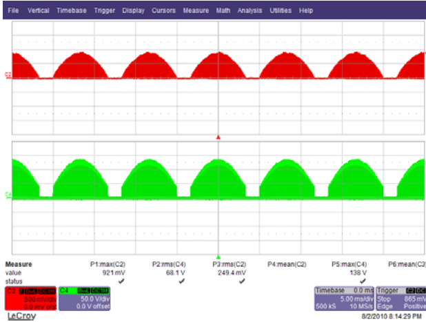
Figure 22 – 90 VAC 60 Hz, Full Load. Upper: I_{DRAIN} , 500 mA / div. Lower: V_{DRAIN} , 50 V, 5 ms / div.
