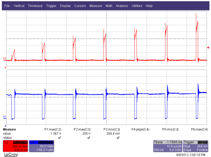
Figure 51 – 132 VAC, 60 Hz Start-up. Upper: I_{DRAIN} , 200 mA / div. Lower: V_{DRAIN} , 50 V, 10 \mu s / div.
