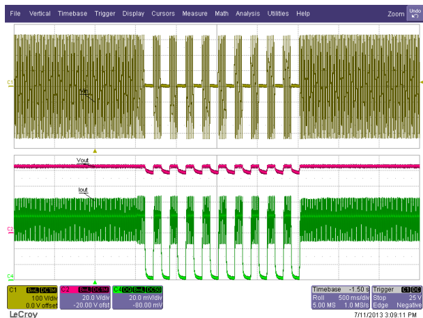
Figure 30 – Line Sag Test at 230 - 0 V at 0.1 Second Interval. Ch1: V_{IN} , 100 V / div. Ch2: V_{OUT} , 20 V / div. Ch4: I_{OUT} , 50 mA / div. Time Scale: 500 ms / div.
