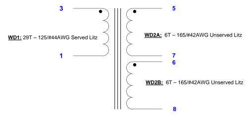
Figure 15 – LLC Transformer Schematic.
