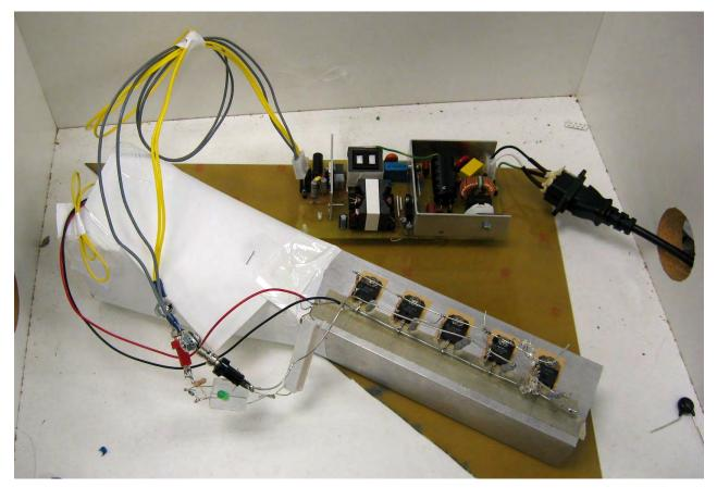
Figure 82 – Line Surge Physical Set-up.
