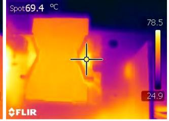
Figure 54 – PFC Inductor (L2), 90 VAC Input, 100% Load, Room Temperature.
