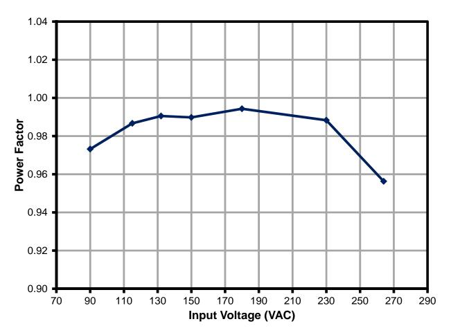
Figure 26 – Power Factor vs. Input Voltage, 100% Load.
