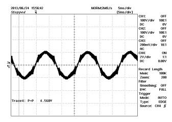
Figure 30 – Input Current, 115 VAC, 150 W Load, 2 A, 5 ms / div.
