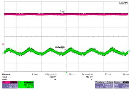
Figure 48 – Output Ripple, Full Load, 115 VAC. Upper: I<sub>OUT</sub>, 1 A / div. Lower: Output Voltage Ripple, 100 mV, 5 ms / div.
