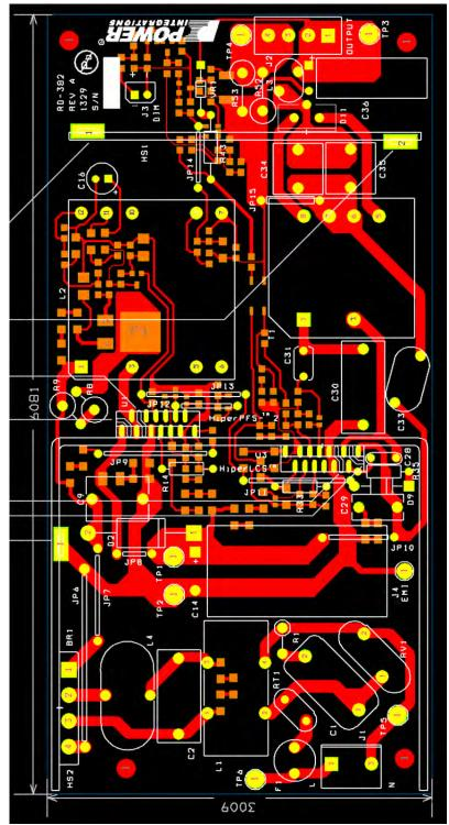
Figure 5 – Printed Circuit Layout, Top Side.
