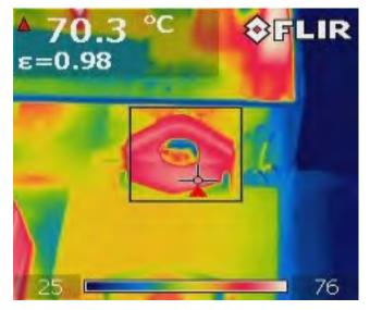
Figure 65 – LLC IC (U3), 115 VAC Input, 100% Load, Room Temperature.
