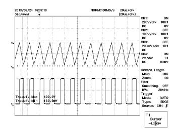
Figure 37 – PFC Stage Drain Voltage and Current, Full Load, 115 VAC. Upper: Switch + Inductor Current, 2 A / div.
