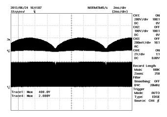
Figure 38 – PFC Stage Drain Voltage and Current, Full Load, 230 VAC. Upper: Switch + Inductor Current, 2 A / div. Lower: V<sub>DRAIN</sub>, 200 V, 2 ms / div.
