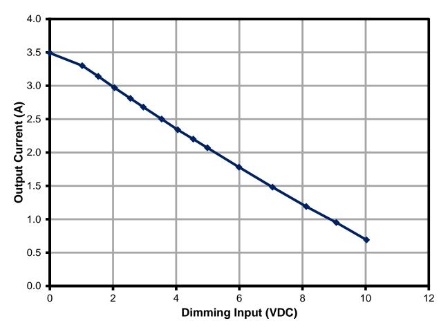
Figure 28 – RD-382 Output Current vs. Dimming Voltage.
