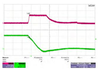
Figure 45 – Output Short-Circuit Test. Upper: LLC I<sub>OUT</sub>, 50 A / div. Lower: LLC V<sub>OUT</sub>, 20 V, 10 μs / div.
