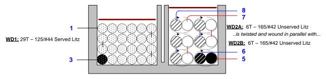
Figure 16 – LLC Transformer Build Diagram.
