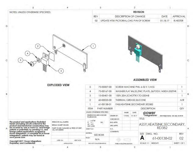
Figure 23 – RD-382 Secondary Heat Sink Assembly.
