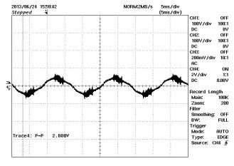
Figure 32 – Input Current, 265 VAC, 150 W Load, 2 A, 5 ms / div.
