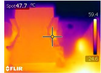
Figure 74 – PFC Inductor (L2), 230 VAC Input, 100% Load, Room Temperature
