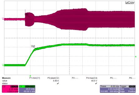
Figure 42 – LLC Start-up. 115 VAC, 100% Load. Upper: LLC Primary Current, 2 A / div. Lower: LLC V<sub>OUT</sub>, 20 V, 2 ms / div.
