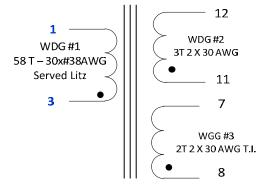
Figure 13 – PFC Choke Electrical Diagram.
