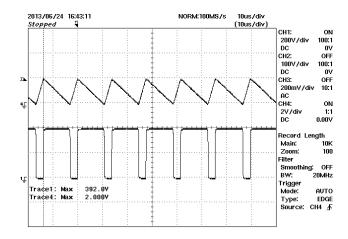
Figure 39 – PFC Stage Drain Voltage and Current, Full Load, 230 VAC. Upper: Switch + Inductor Current, 2 A / div. Lower: V<sub>DRAIN</sub>, 200 V, 10 μs / div.
