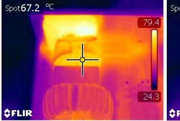
Figure 61 – Differential Mode Choke (L4), 115 VAC Input, 100% Load, Room Temperature.
