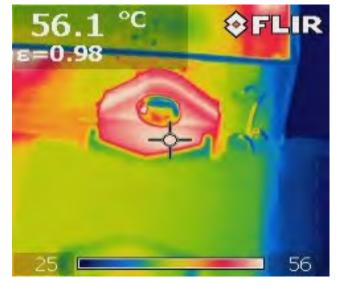
Figure 75 – LLC IC (U3), 230 VAC Input, 100% Load, Room Temperature.
