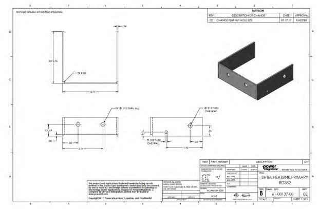
Figure 18 - RD-382 Primary Heat Sink Sheet Metal Drawing.
