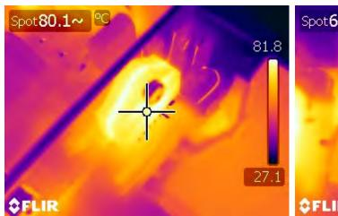
Figure 53 – PFC IC (U1), 90 VAC Input, 100% Load, Room Temperature.
