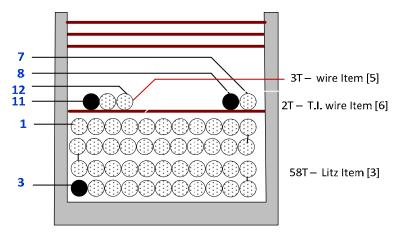
Figure 14 – PFC Inductor Build Diagram.
