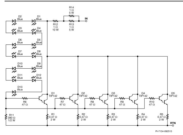
Figure 10 – Constant Voltage Load Schematic.
