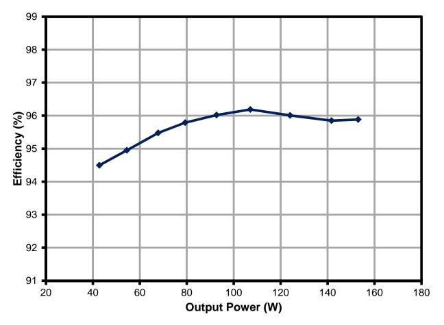
Figure 24 – LLC Stage Efficiency vs. Load, 380 VDC Input.
