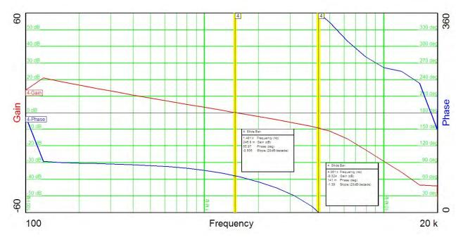
Figure 79 – LLC Converter Gain-Phase, 100% Load Crossover Frequency – 1.5 kHz, Phase Margin - 66°.
