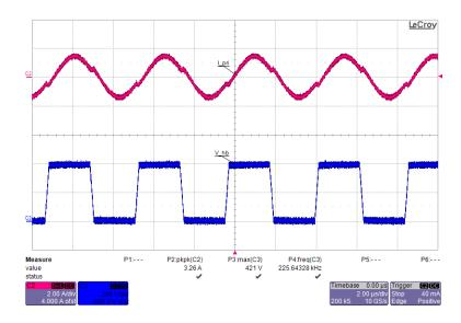
**Figure 33** – LLC Stage Primary Voltage and Current, 100% Load. Upper: Current, 2 A / div. Lower: Voltage, 200 V, 2 μs / div.
