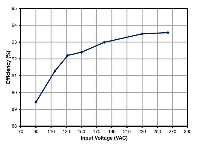
Figure 25 – Total Efficiency vs. Input Voltage, 100% Load.
