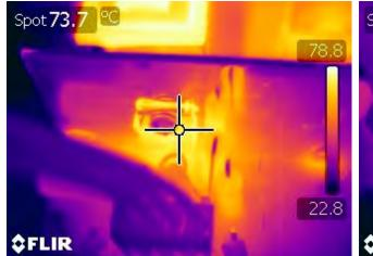
Figure 57 – Output Rectifier (D11), 90 VAC Input, 100% Load, Room Temperature.
