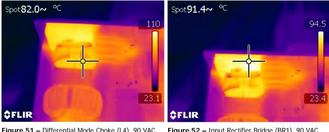
Figure 51 – Differential Mode Choke (L4), 90 VAC Input, 100% Load, Room Temperature.
