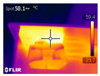
Figure 72 – Input Rectifier Bridge (BR1), 230 VAC Input, 100% Load, Room Temperature.
