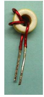
Figure 16 – Finished Part, Front View. Tin Leads to within ~ 1/8" of Toroid Body.
