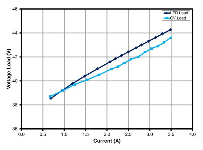
Figure 12 – Comparison of Streetlight LED Array V-I Characteristic with CV Load.
