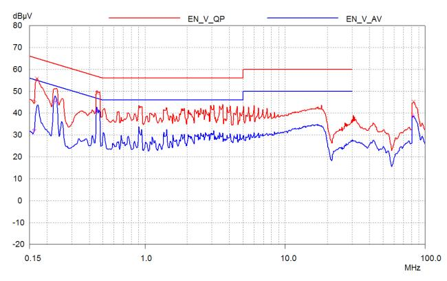
Figure 81 – Conducted EMI, 230 VAC, Full Load.
