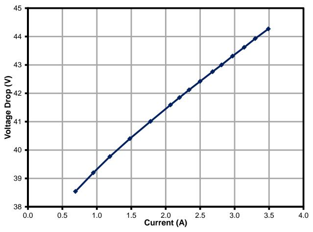
Figure 7 – Streetlight LED Array V-I Characteristic.
