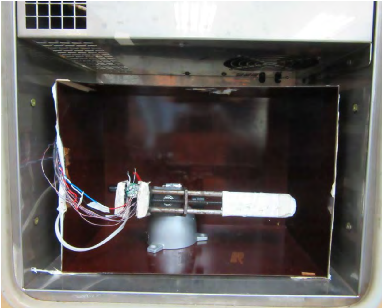
Figure 46 – Test Set-up Picture Thermal at 85 °C Ambient - Open Frame.
