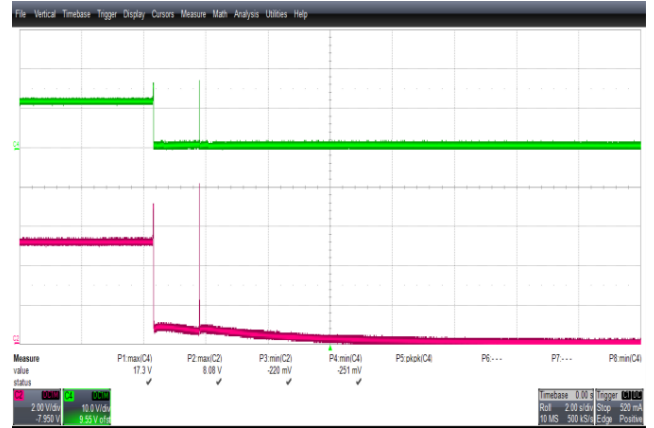
Figure 43 – Output Voltage Waveform. 265 VAC Input. Upper: 12 V, 10 V / div. Lower: 5 V, 2 V / , 2 s / div.
