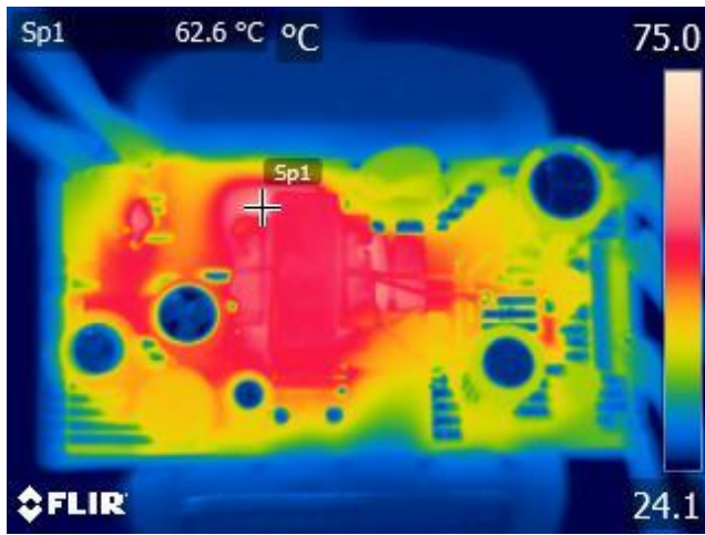
Figure 18 – Transformer Side. 90 VAC, Full Load.
