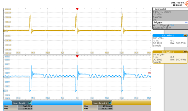
Figure 32 – 265 VAC Input. Condition: 3.8 V – 20 mA, 12 V – 20 mA. Upper: I_{DRAIN} , 50 mA / div. Lower: V_{DRAIN} , 100 V / div., 5 \mu s / div.
