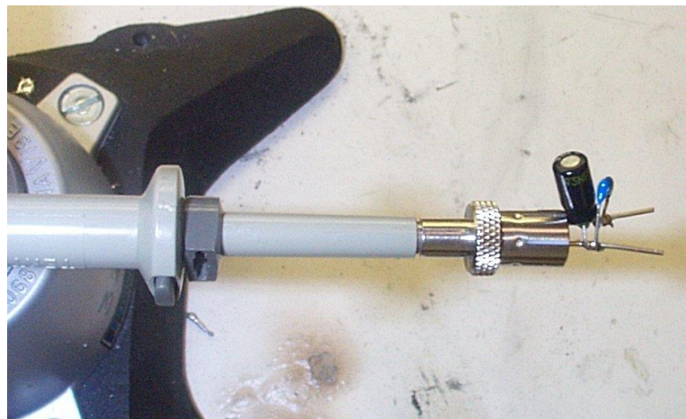
Figure 90 – Oscilloscope Probe with Probe Master ( www.probemaster.com ) 4987A BNC Adapter. (Modified with wires for ripple measurement, and two parallel decoupling capacitors added)
