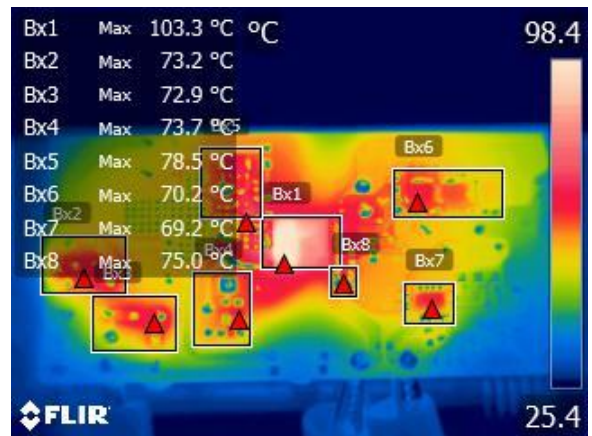
Figure 44 – Bottom Components, Ambient = 27 °C.
