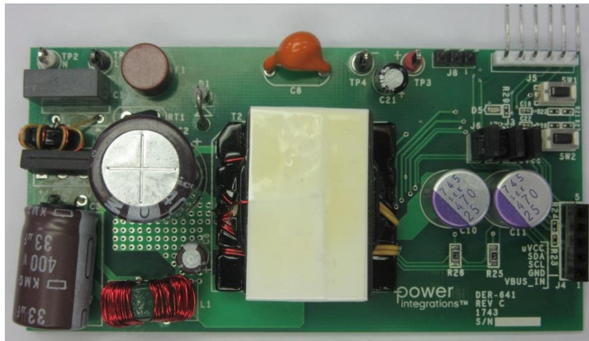
Figure 1 – Populated Circuit Board Photograph, Top. (DER-641 is equivalent to RD-641.)
