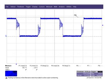
**Figure 43** – Output Rectifier (D11) Reverse Voltage, 100% Load. 20 V, 2 μs / div.
