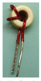
**Figure 17** – Finished Part, Front View. Tin Leads to within  $\sim 1/8"$  of Toroid Body.
