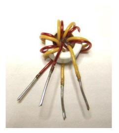
**Figure 19** – Finished Inductor.
