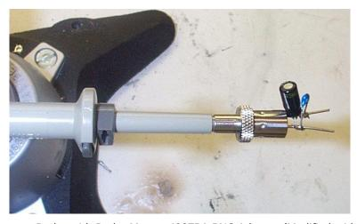
**Figure 58** — Oscilloscope Probe with Probe Master 4987BA BNC Adapter (Modified with Wires for Probe Ground for Ripple measurement and Two Parallel Decoupling Capacitors Added).
