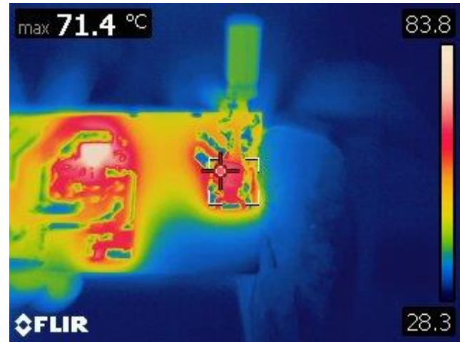
Figure 40 – D3 – Output Diode. Spot: 71.4 °C.
