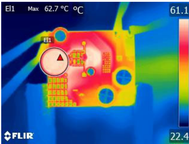
Figure 12 – Buck Choke (EI1), 62.7 °C. 85 VAC, 800 mA Output.
