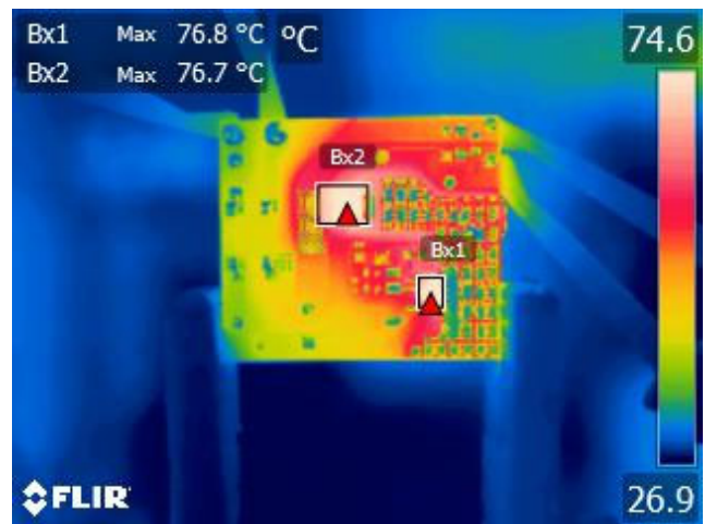
Figure 15 – LNK3209D (Bx1), 76.8 °C. Buck Diode (Bx2), 76.7 °C. 265 VAC, 800 mA Output.
