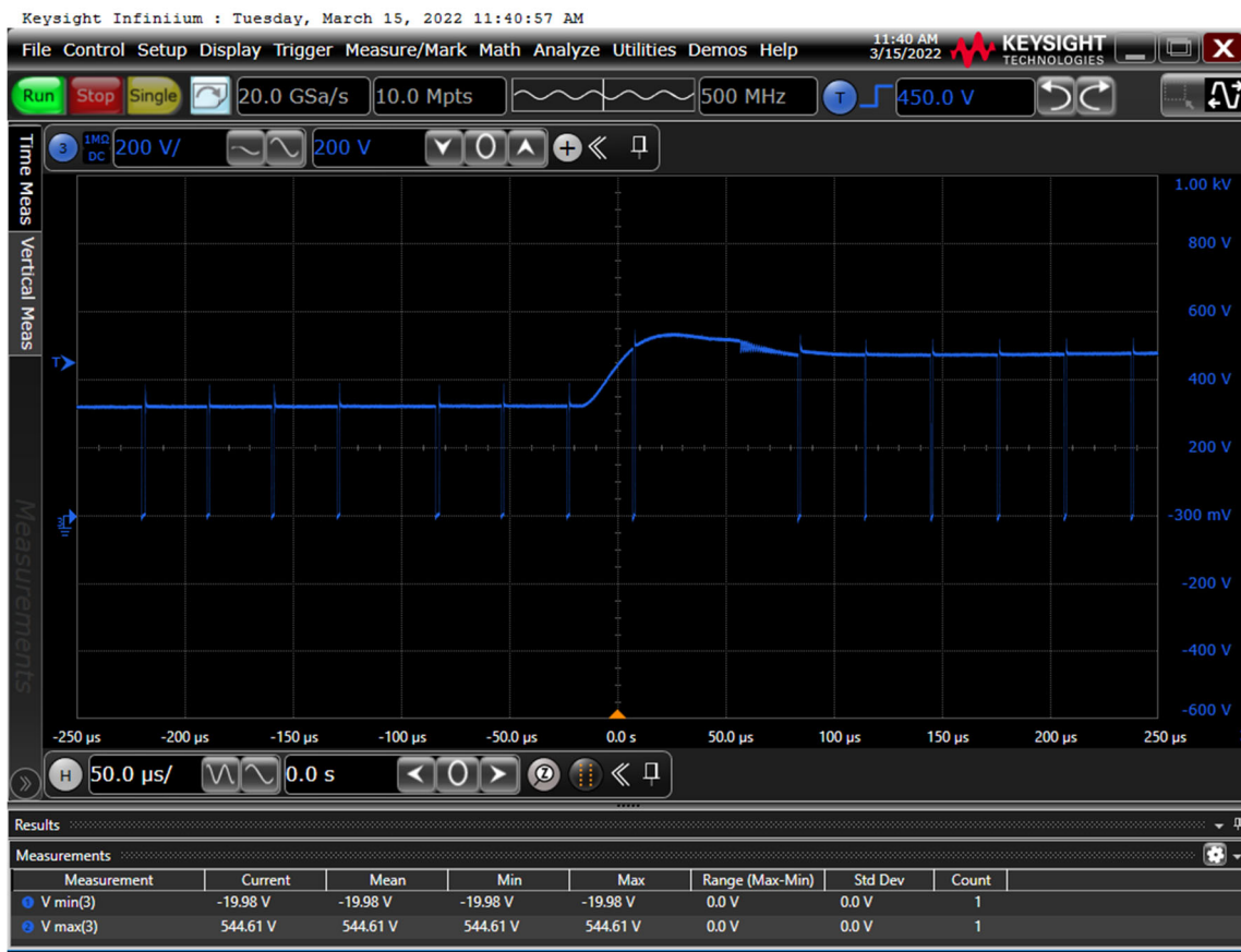
Figure 97 – Drain Voltage, 230 VAC, Full Load.
