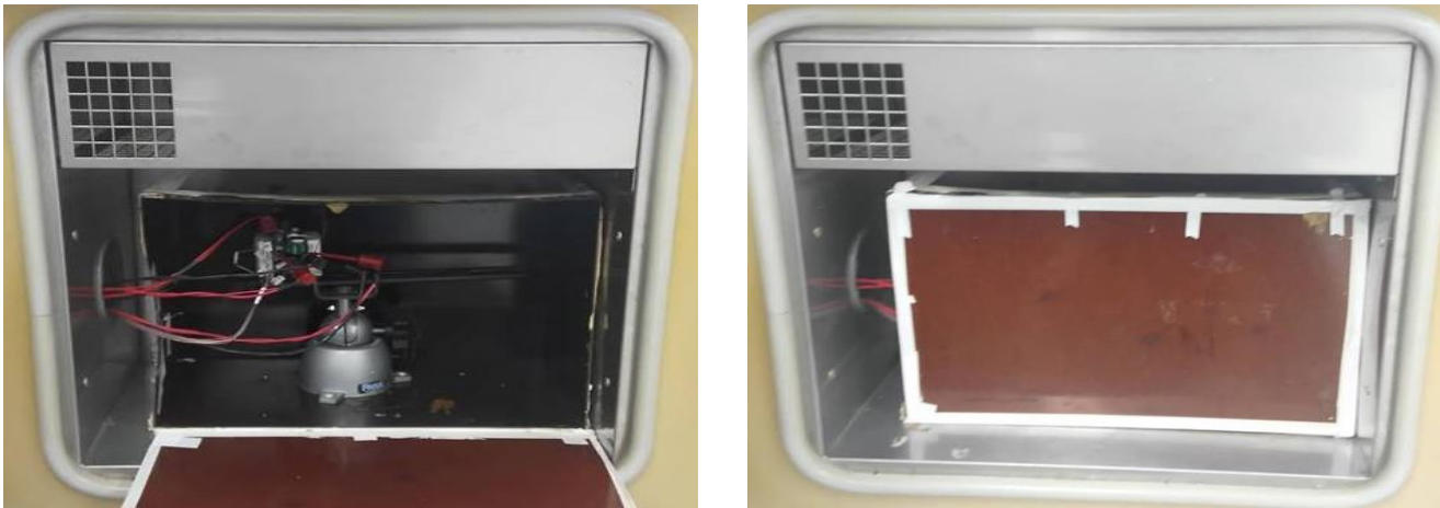
Figure 74 – Thermal Performance Set-up Using Thermal Chamber.
