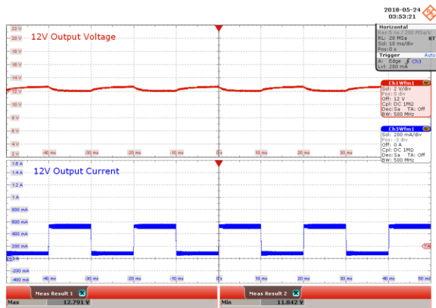
Figure 59 – 85 VAC Input. Upper: 12 V V_{OUT} , 2 V / div., 10 ms / div. Lower: 12 V I_{OUT} , 200 mA / div. V_{MAX} : 12.791 V. V_{MIN} : 11.842 V.
