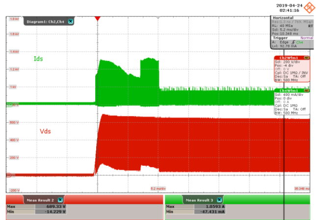
Figure 17 – Drain Voltage and Current Waveforms. 440 VAC, 120 mA Output. Upper: I_{DRAIN} , 400 mA / div. Lower: V_{DRAIN} , 200 V, 5.2 ms / div. I_{MAX} = 1.0593 A, V_{MAX} = 689.3 V
