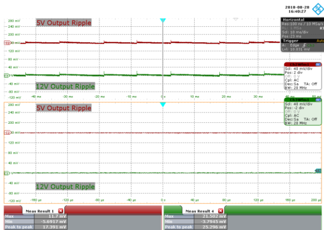
Figure 126 – 85 VAC 60 Hz, 0% Load. CH2: 5 V OUT , 40 mV / div., 10 ms / div. CH3: 12 V OUT , 40 mV / div., 10 ms / div. Zoom: 40 μs / div. 5 V Output Ripple = 17.391 mV. 12 V Output Ripple = 25.296 mV.
