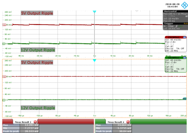
Figure 126 – 85 VAC 60 Hz, 0% Load. CH2: 5 V OUT , 40 mV / div., 10 ms / div. CH3: 12 V OUT , 40 mV / div., 10 ms / div. Zoom: 40 μs / div. 5 V Output Ripple = 17.391 mV. 12 V Output Ripple = 25.296 mV.
