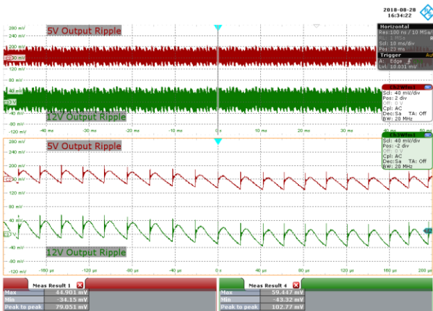
Figure 114 – 85 VAC 60 Hz, 75% Load. CH2: 5 V OUT , 40 mV / div., 10 ms / div. CH3: 12 V OUT , 40 mV / div., 10 ms / div. Zoom: 40 μs / div. 5 V Output Ripple = 112.25 mV. 12 V Output Ripple = 131.23 mV.
