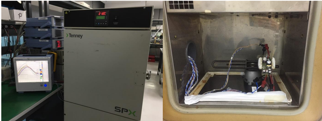
Figure 147 – Thermal Performance Set-up using Thermal Chamber.
