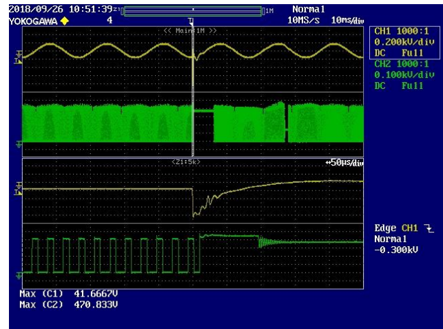
Figure 131 – (-)1 kV Differential Surge, 270° Phase Angle. Lower: V_{DRAIN} , 100 V / div., 10 ms / div. Peak V_{DRAIN} : 470.83 V.
