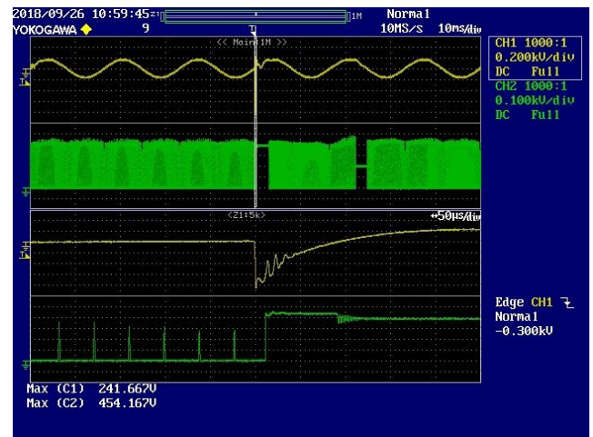
Figure 129 – (-)1 kV Differential Surge, 0° Phase Angle. Lower: V_{DRAIN} , 100 V / div., 10 ms / div. Peak V_{DRAIN} : 454.17 V.
