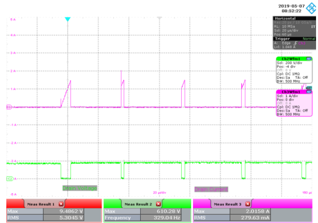
Figure 90 – 100 VAC, 48 V LED Load. Upper: I_{DRAIN} , 1 A / div. Lower: V_{DRAIN} , 200 V / div., 20 μs / div.
