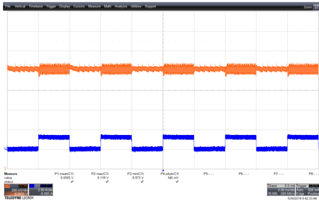
Figure 79 – Transient Response. 90 VAC, 9 V, 0 – 1.25 A Load Step. V_{MIN} : 8.973 V, V_{MAX} : 9.119 V. Upper: V_{OUT} , 0.2 V / div., 5 ms / div. Lower: I_{LOAD} , 2 A / div.
