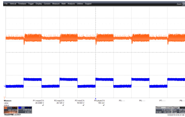
Figure 96 – Transient Response. 265 VAC, 20 V, 0 – 1.25 A Load Step. V_{MIN} : 19.933 V, V_{MAX} : 20.125 V. Upper: V_{OUT} , 0.2 V / div., 5 ms / div. Lower: I_{LOAD} , 2 A / div.
