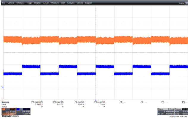
Figure 67 – Transient Response. 90 VAC, 3.3 V, 2.5 – 3.75 A Load Step. V_{MIN} : 3.24 V, V_{MAX} : 3.412 V. Upper: V_{OUT} , 0.2 V / div., 5 ms / div. Lower: I_{LOAD} , 2 A / div.
