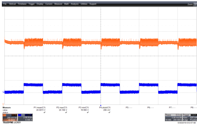
Figure 95 – Transient Response. 90 VAC, 20 V, 0 – 1.25 A Load Step. V_{MIN} : 19.9 V, V_{MAX} : 20.106 V. Upper: V_{OUT} , 0.2 V / div., 5 ms / div. Lower: I_{LOAD} , 2 A / div.
