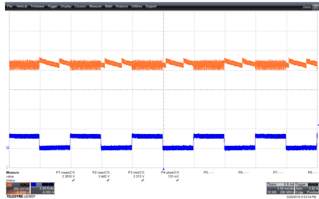
Figure 64 – Transient Response. 265 VAC, 3.3 V, 0 – 1.25 A Load Step. V_{MIN} : 3.313 V, V_{MAX} : 3.445 V. Upper: V_{OUT} , 0.2 V / div., 5 ms / div. Lower: I_{LOAD} , 2 A / div.
