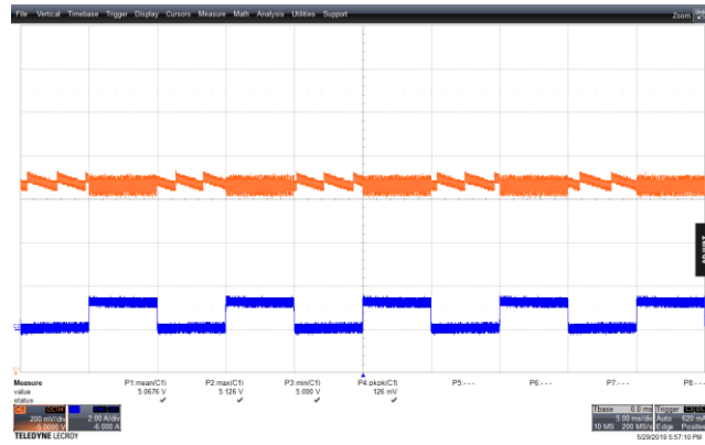
Figure 72 – Transient Response. 265 VAC, 5 V, 0 – 1.25 A Load Step. V_{MIN} : 5 V, V_{MAX} : 5.126 V. Upper: V_{OUT} , 0.2 V / div., 5 ms / div. Lower: I_{LOAD} , 2 A / div.
