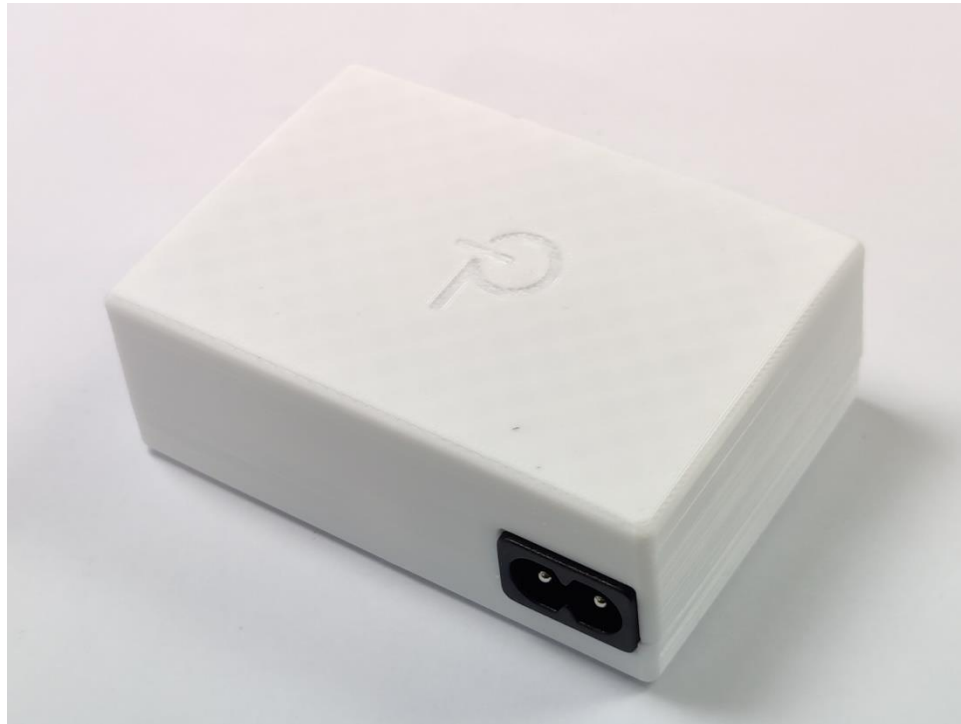
Figure 4 – Enclosed Power Supply Unit Photograph.
