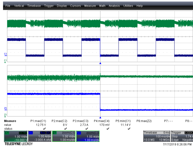
Figure 102 – Output Load Transient, 100% to 0% Load.
