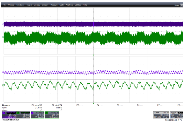
Figure 113 – 90 VAC 60 Hz, Full Load Normal. Upper: V_{USB-A} , 50 mV / div., 10 ms / div. Lower: V_{USB-C} , 50 mV / div. V_{RIPPLE(USB-A)} = 21.3\text{ mVpp} . V_{RIPPLE(USB-C)} = 133\text{ mVpp} .
