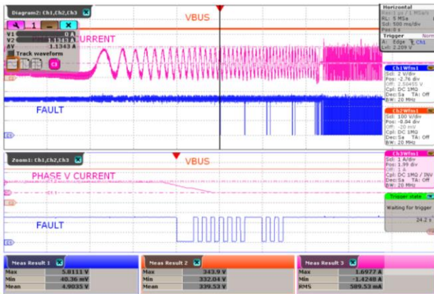
Figure 45 – OCP at R_{XL}/R_{XH} = 115\text{ k}\Omega , I_{LIM} = 1\text{ A} . CH2: V_{BUS} , 100 V / div. CH3: I_{PHASE} , 1 A / div. CH1: V_{FAULT} , 2 V / div. Time Scale: 500 ms / div. Time Scale (Zoomed Area): 100 \mu s / div. FAULT Flag Reading = 0000010.
