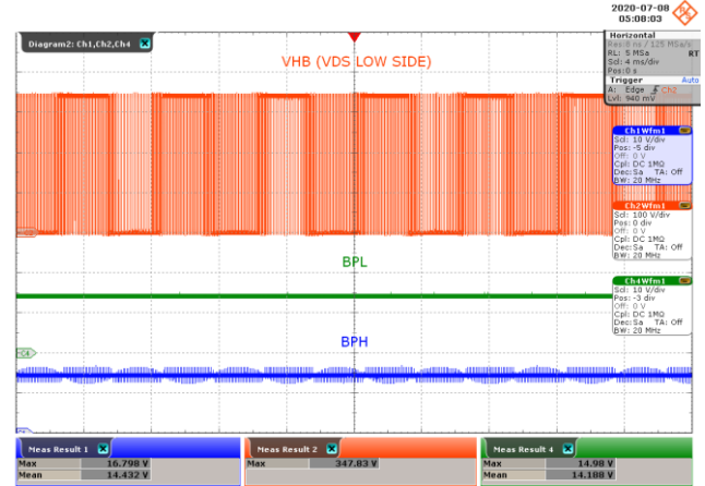
Figure 35 – BPL and BPH Signal at 200W Load. CH2: V_{HB\_PHASEW} , 100 V / div. CH4: V_{BPL} , 10 V / div. CH1: V_{BPH} , 10 V / div. Time Scale: 4 ms / div. BPL Average Voltage = 14.18 V. BPH Average Voltage = 14.43 V.
