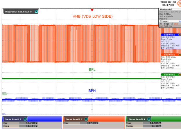
Figure 34 – BPL and BPH Signal at 100W Load. CH2: V_{HB\_PHASEW} , 100 V / div. CH4: V_{BPL} , 10 V / div. CH1: V_{BPH} , 10 V / div. Time Scale: 4 ms / div. BPL Average Voltage = 14.18 V. BPH Average Voltage = 14.44 V.
