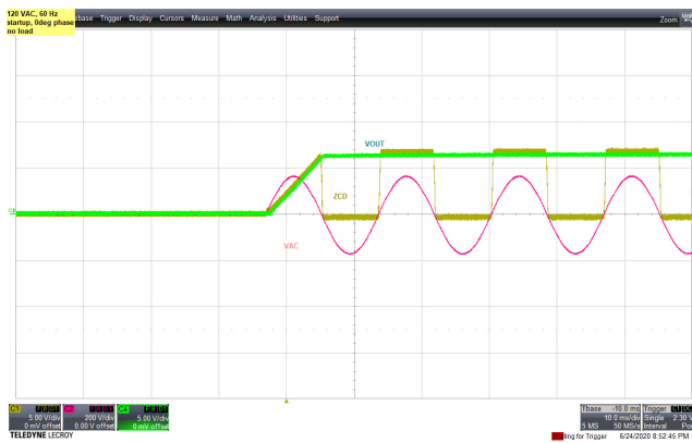
Figure 14 – 120 VAC 60 Hz, No-Load. CH1: ZCD, 5 V / div., 5 ms / div. CH2: V_{IN} , 100 V / div., 5 ms / div. CH4: V_{OUT} , 5 V / div., 5 ms / div.
