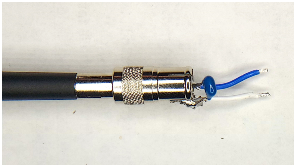
Figure 43 – Oscilloscope Probe with Probe Master ( www.probemaster.com ) 4987A BNC Adapter. (Modified with wires for ripple measurement, and one parallel decoupling capacitor added)
