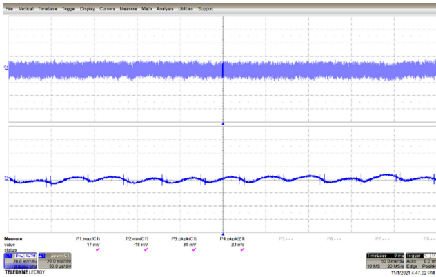
Figure 56 – Output Voltage Ripple. V_{IN} = 300 \text{ VDC} , I_{OUT} = 0.625 \text{ A} . Upper: V_{OUT} , 20 mV, 50 ms / div. Lower: Zoom @ 50 \mu\text{s} / div. V_{RIPPLE} = 34 \text{ mV}_{P-P} .
