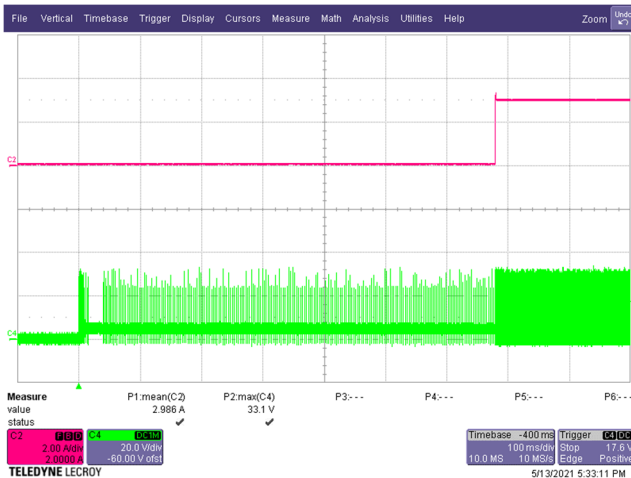
Figure 26 – SR FET Drain Voltage and Load Current. 90 VAC, 5.0 V, 3 A Load (33.1 V MAX ). C4: V DRAIN(SR) , 20 V / div. C2: I Load , 2 A / div. Time: 100 ms / div.
