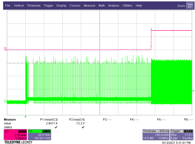
Figure 27 – SR FET Drain Voltage and Load Current. 265 VAC, 5.0 V, 3 A Load (72.2 V MAX ). C4: V DRAIN(SR) , 20 V / div. C2: I Load , 2 A / div. Time: 100 ms / div.
