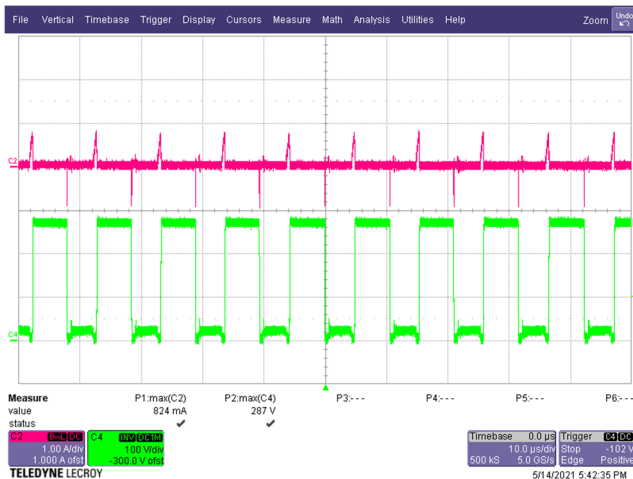
Figure 50 – Primary Clamp Drain Voltage and Current. 90 VAC, 20.0 V, 3 A Load (287 V MAX ). C4: V DRAIN , 100 V / div. C2: I DRAIN , 1 A / div. Time: 10 μs / div.
