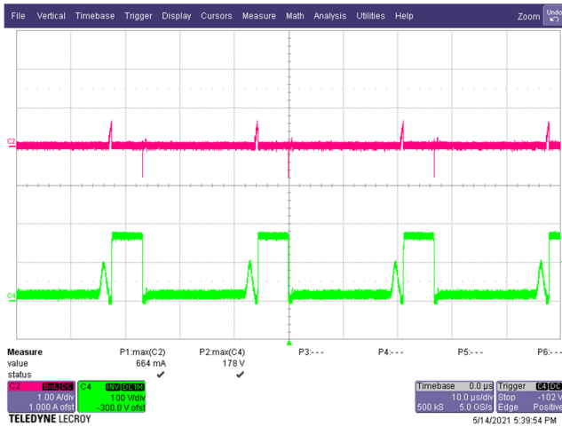
Figure 44 – Primary Clamp Drain Voltage and Current. 90 VAC, 5.0 V, 3 A Load (178 V MAX ). C4: V DRAIN , 100 V / div. C2: I DRAIN , 1 A / div. Time: 10 μs / div.
