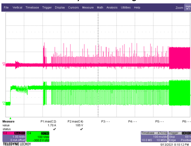
Figure 22 – Primary Drain Voltage and Current. 90 VAC, 5.0 V, 3 A Load (185 V MAX ). C4: V DRAIN , 100 V / div. C2: I DRAIN , 1 A / div. Time: 100 ms / div.
