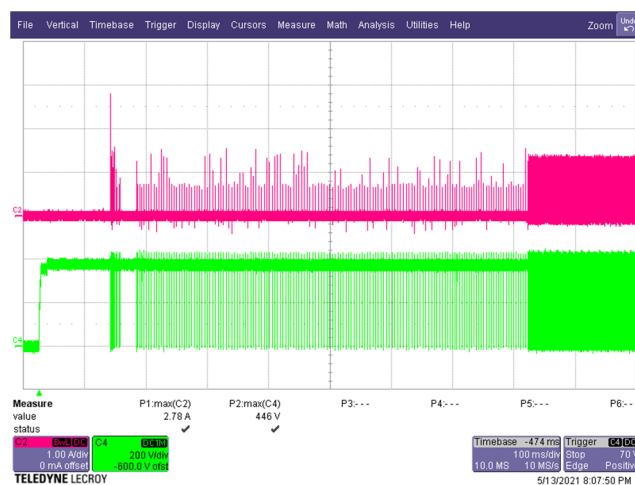
Figure 23 – Primary Drain Voltage and Current. 265 VAC, 5.0 V, 3 A Load (446 V MAX ). C4: V DRAIN , 200 V / div. C2: I DRAIN , 1 A / div. Time: 100 ms / div.
