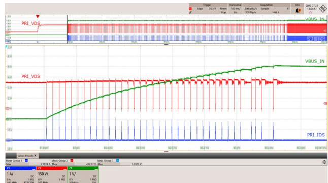
Figure 36 – Primary Drain Voltage and Current. 265 VAC, 5.0 V, 3 A (E-load CR Mode, 1.63 Ω at the End of 100 mΩ Cable). V_{DS\_PRI} = 452.37 V Maximum. CH1: I_{DS\_PRI} , 1 A / div. CH2: V_{DS\_PRI} , 150 V / div. CH3: V_{BUS\_IN} , 1 V / div. Time: 100 ms / div. (200 μs / div. Zoom).
