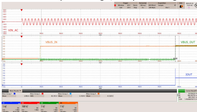
Figure 33 – Input Voltage, Output Voltage and Current. 90 VAC, 5.0 V, 3 A (E-load CC Mode). V_{BUS\_IN} = 5.143 V Steady-State. t_{output\_delay} = 780 ms CH1: IOUT, 1 A / div. CH2: V_{IN\_AC} , 100 V / div. CH3: V_{BUS\_OUT} , 1 V / div. CH4: V_{BUS\_IN} , 1 V / div. Time: 100 ms / div.
