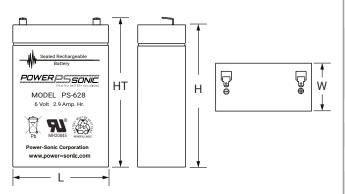
**W:** 1.30 (33) **H:** 3.86 (98) **HT:** 4.06 (103) **L:** 2.60 (66) Tolerances are +/- 0.04 in. (+/- 1mm) and +/- 0.08 in. (+/- 2mm) for height dimensions.
