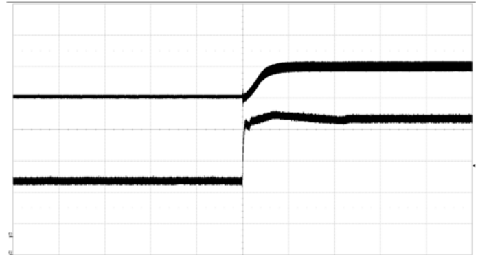
HRR product output at input voltage step 36-75 V, 1 ms/div Bottom trace – input voltage change 36-75 V, 20 V/div Top trace – resulting output voltage change, 1 V/div
